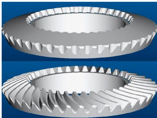
6 Crown gear with pressed chamfers
