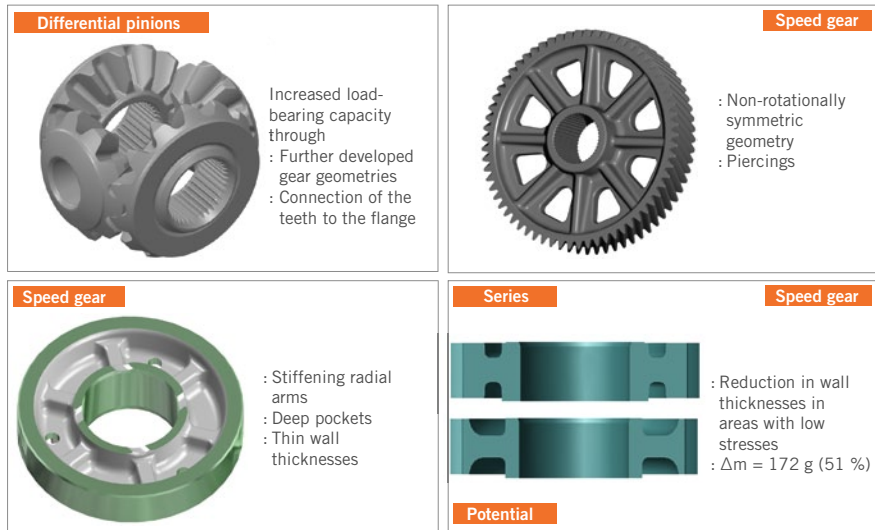
⑦ Lightweight design potential on transmission parts (Sources: Metaldyne, metallumform, Seissenschmidt, Sona BLW Präzisionsschmiede)
